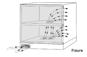
System 4 is completely automatic; fan operation and speed is controlled by the temperature within the enclosure.
